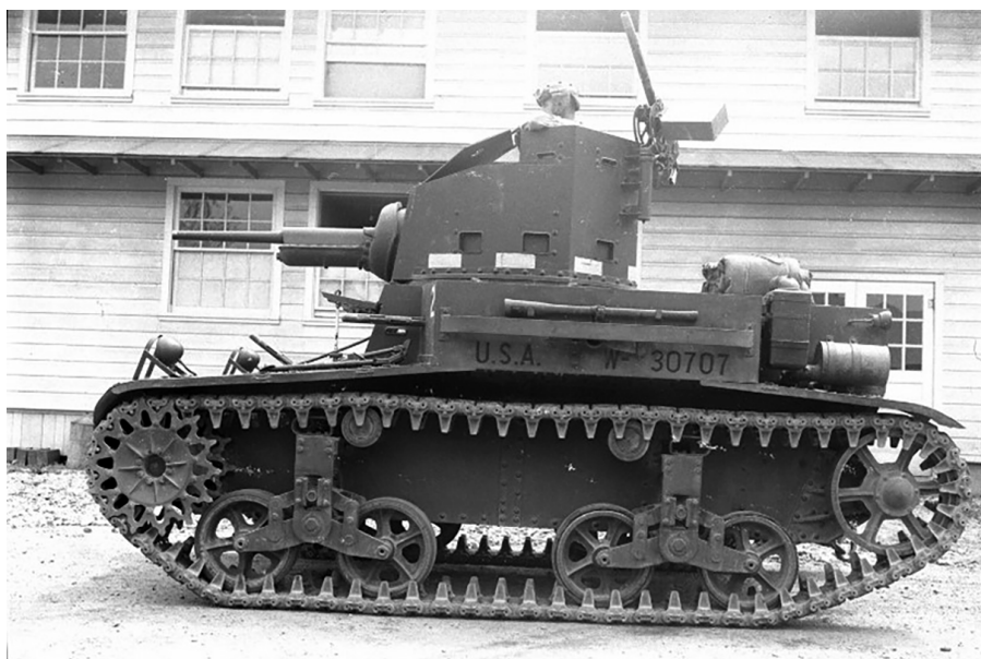
Figure 2. The M2A4 Light Tank with a turret-mounted 37mm gun. (U.S. Army Armor and Cavalry Collection)
