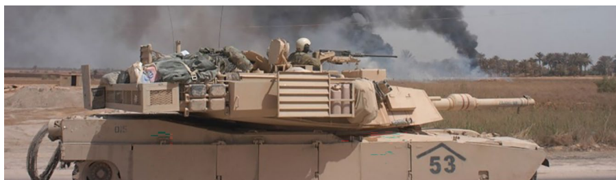
Figure 9. An M1A1 of the 3 rd Infantry Division during Operation Iraqi Freedom I. The extended bustle rack was fabricated before the invasion began when it became clear that division combat units would need more supplies than their trains could accommodate. (U.S. Army Armor School Branch Archives)
