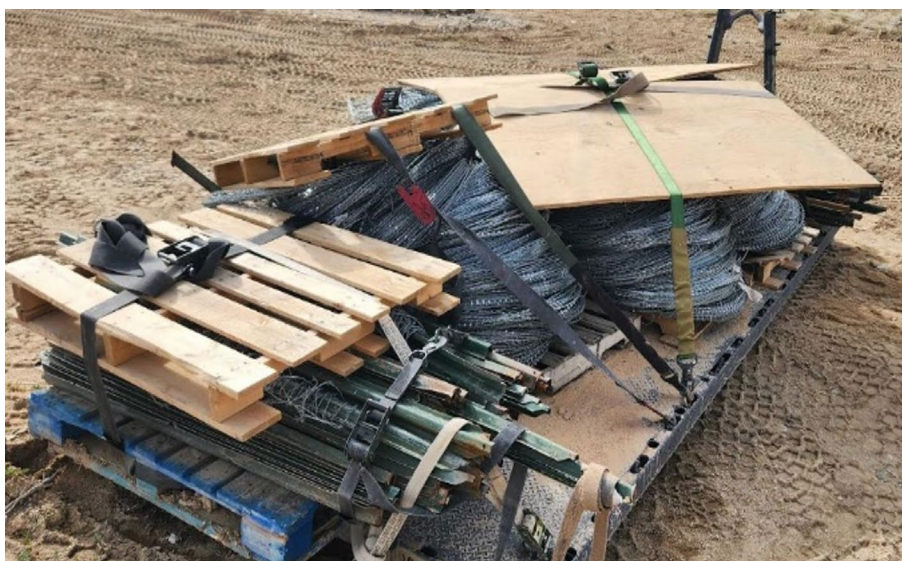
Figure 1. Poorly built CCL loaded with concertina wire, pickets, and barbed wire. Note the Concertina Wire falling over and randomly placed ratchet straps. (U.S. Army photo by CPT Olivia Schretzman and MAJ William Longwell)
